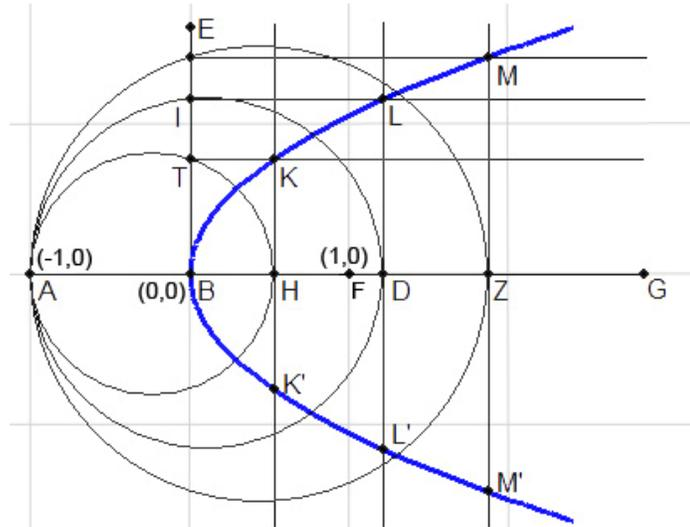
$(x-2)^2 = 8(y-1)$ , with focus F, vertex B, parameter AB (=2)
